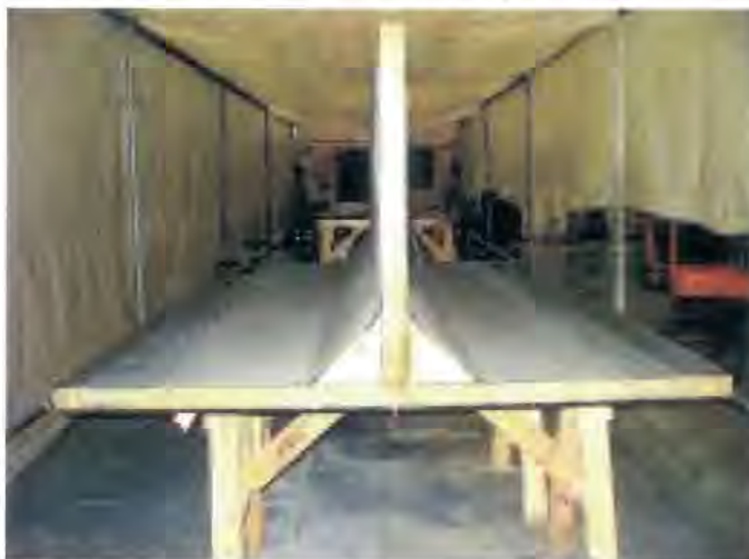
Figure 4 – Simple 2D Joint Specimen
