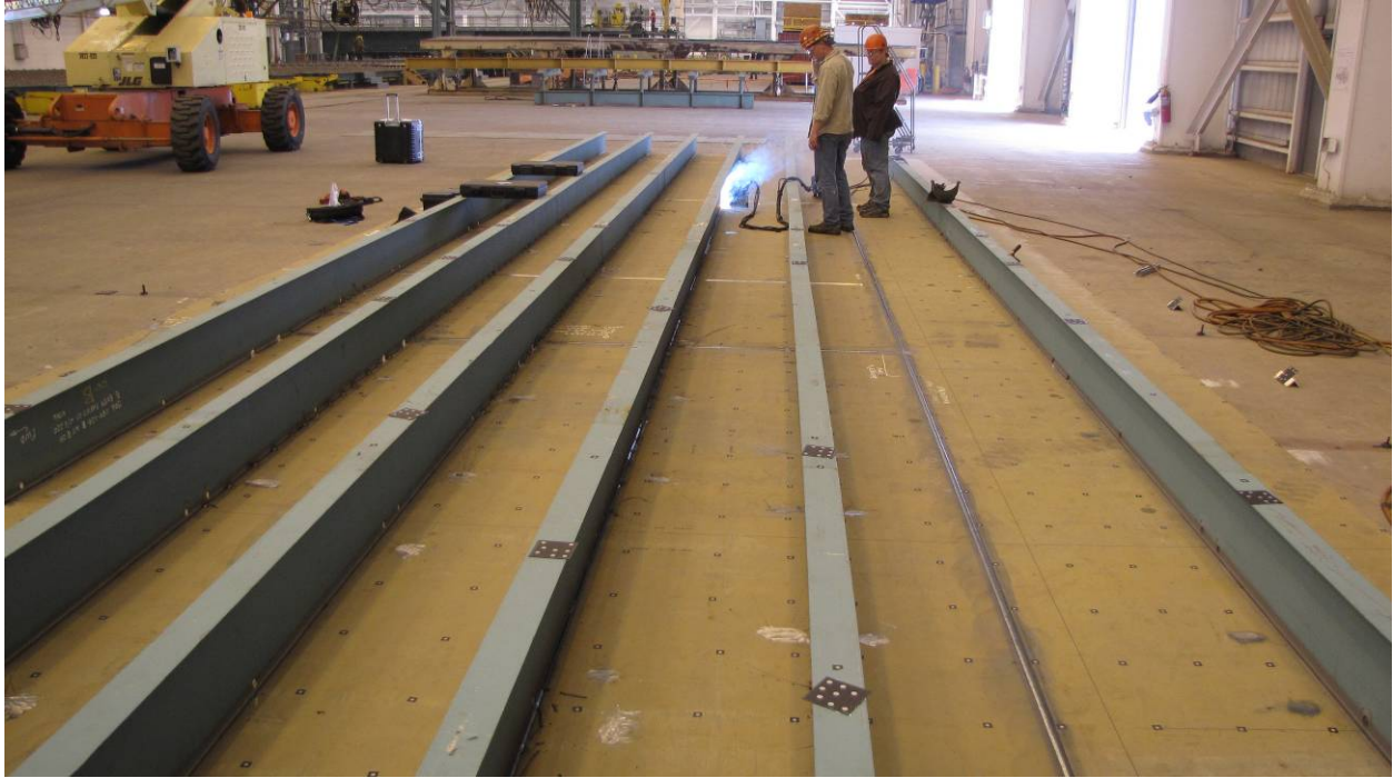
Figure 7. Targeting required for Real Time Photogrammetry
