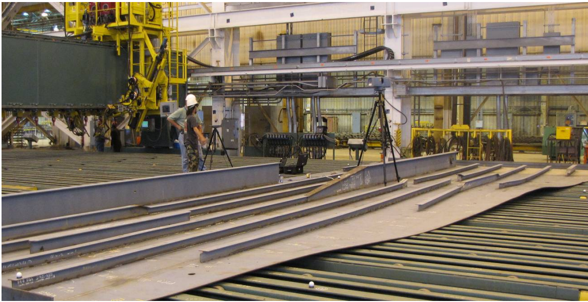
Figure 9. Surphaser Laser Scanner Surveying Plate with Structure
