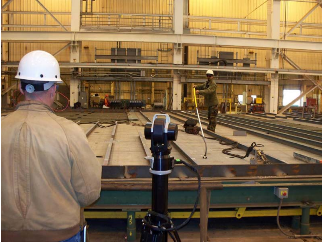
Figure 3. API Laser Tracker 3 Measurements on Panel Line
