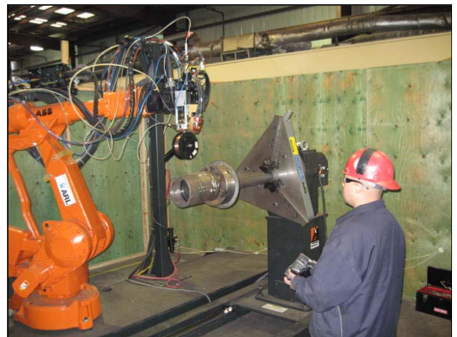
Figure 19. Photograph showing the operator jogging the robot to teach the approximate joint location.
