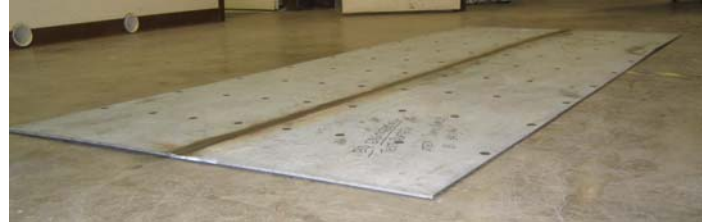
Figure 2. Photograph of the hybrid welded panel.
