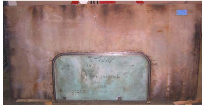
Figure 5. Photograph of 2 by 4 foot insert (AB/EH36, T=10 mm) hybrid laser arc welding into a 4 by 8 foot panel (AB/DH36, T=5 mm).
