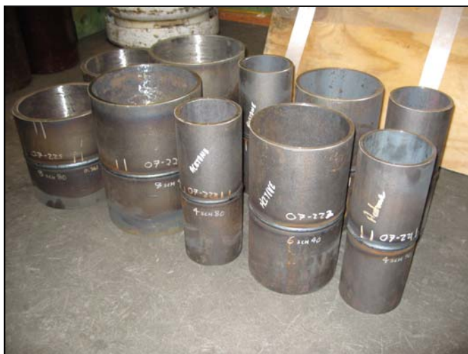
Figure 20. Photograph of pipes joined with a hybrid laser-GMA weld for the small production test run time study.
