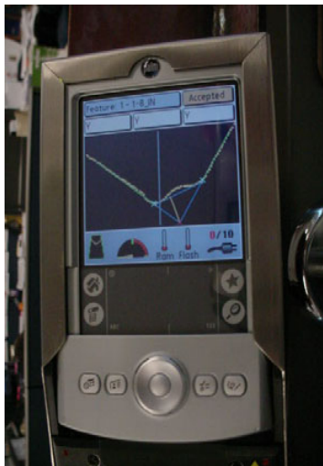
Figure 11 Unit working with weld profile shown
