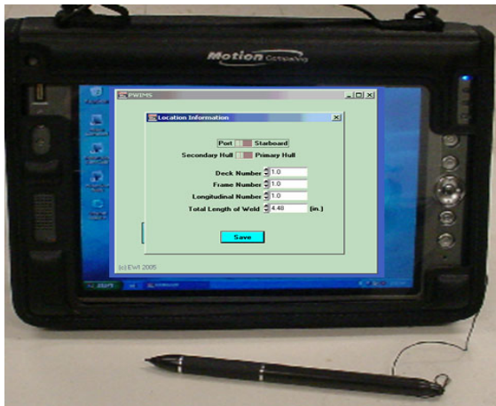
Figure 5 Tablet GUI developed for collecting, reviewing, and augmenting inspection data
