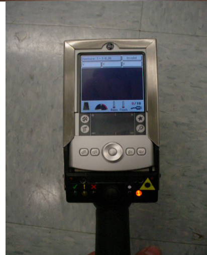
Figure 2 Servo-Robot commercial weld profile laser sensor
