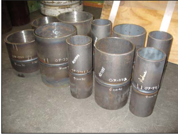
Figure 22. Photograph of pipes joined with a hybrid laser-GMA weld for the small production test run time study.
