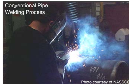
Figure 1. Photograph of the conventional pipe welding process.
