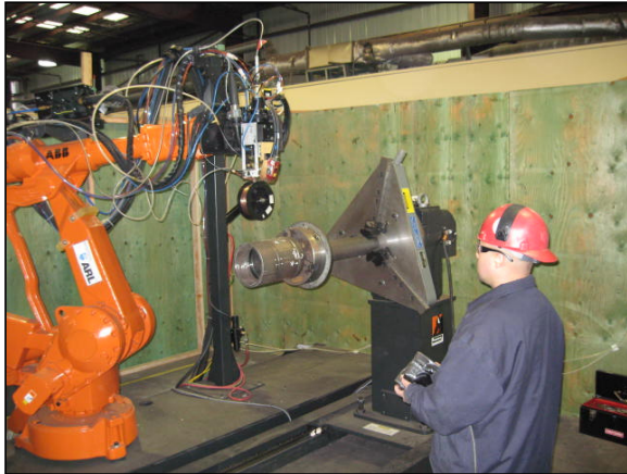
Figure 4. Photograph showing the operator jogging the robot to teach the approximate joint location.
