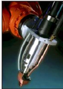
A hybrid laser/GMAW pipe welding system will provide radiographic-quality welds in one or two passes.
