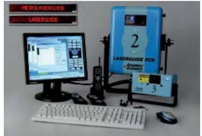
Image Projection hardware, including Marquis Billboard (upper left), projectors (#2 and #3) and personal computer.
