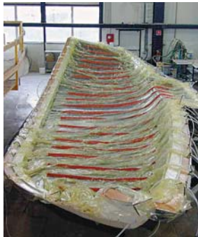
Left and Center: Examples of composite structures during the resin infusion process.
