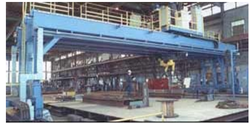
Electric Boat's Programmable Automated Welding System (PAWS).
